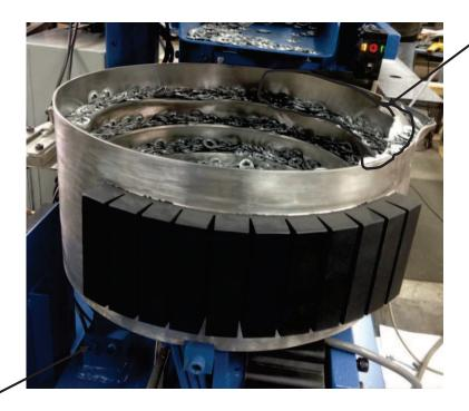
POSSIBLE BROKEN SPRING OR LOOSE FASTENER
